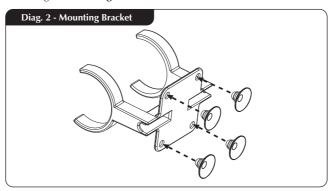
2. Push the the Mounting Bracket on to the body of the skimmer. It can be located anywhere on the height of the skimmer and should be set according to position of the skimmer inside your aquarium (diagram 3).
